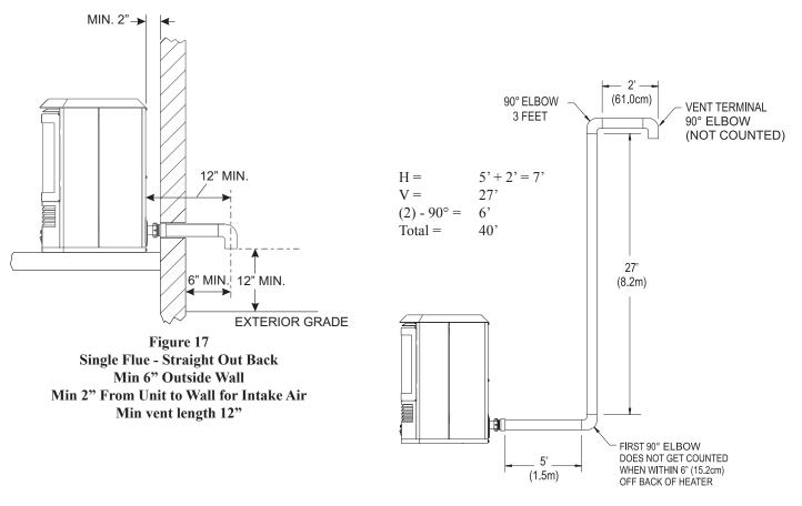
Figure 18 Single Flue - Horizontal Tall Vent Run Example Calculation Max Vent Run 40'
